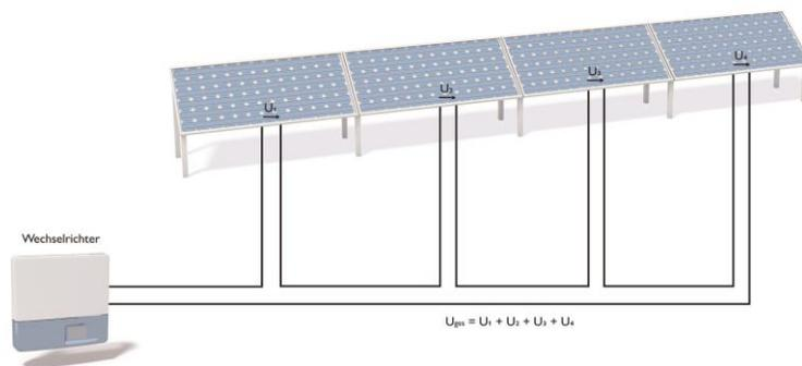
**Figure 1** - Diagram of a typical solar power system: The serial linking of the solar modules means a build-up of system voltage to several hundred volts.
