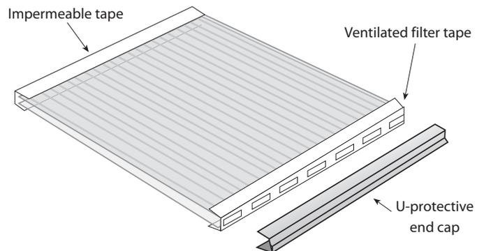
**Figure 17c.** Installation of Impermeable Tape at Top of the Sheet and
