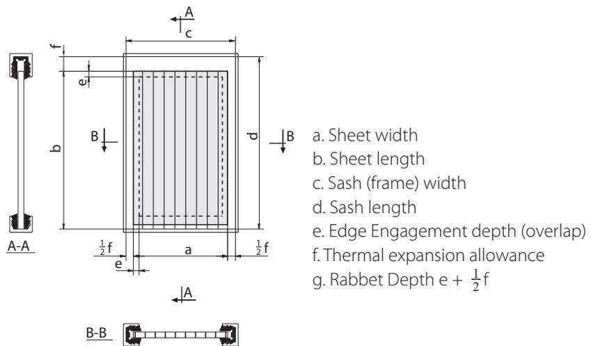
Figure 16c. Schematic Sketch of Rabbet depth and Expansion Allowance. ("wet" and "dry" methods)
