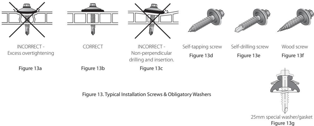
Figure 13. Typical Installation Screws & Obligatory Washers
