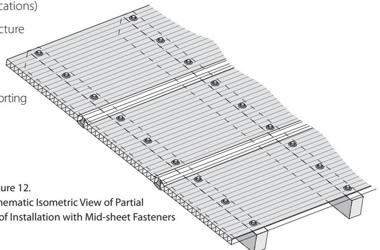
Figure 12. Schematic Isometric View of Partial Roof Installation with Mid-sheet Fasteners
