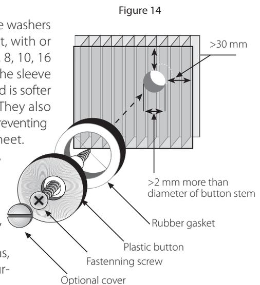
PALRAM recommends perforating SUNLITE for fastening as little as possible, and prefers the use of clamped edge installation. PALRAM recommends that the use of fastening screws in a glazing system, even with plastic buttons, should be limited to economical, price conscious projects only. Two or four-sided clamped glazing is a preferred choice.
